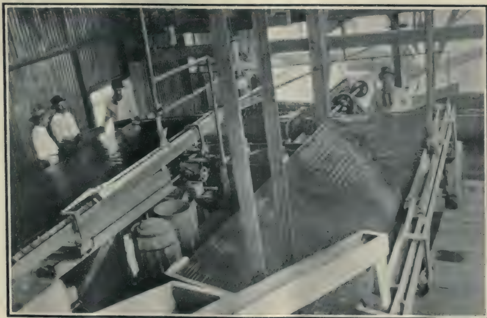
WOLFRAM DRESSING FLOORS AT PISCO-YACU: WILFLEYS, FRUE VANNERS, AND ROUND BUDDLES
